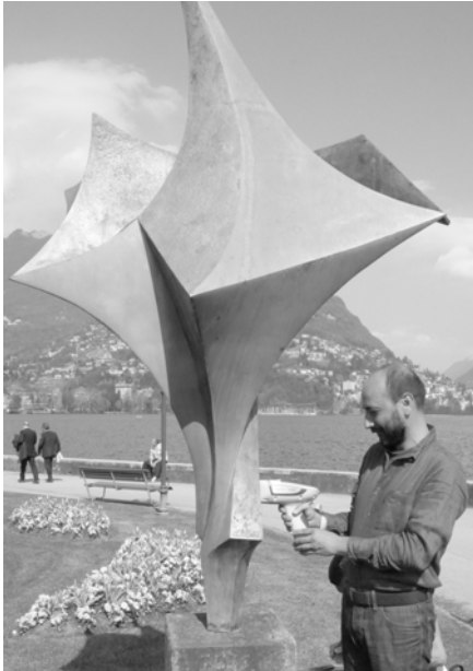
Fig. 11. Portable XRF being used to identify elements present in metal sculptures, in this case Composizione by Bruno Morenzoni, 1983. This sculpture was described as aluminium in the literature, but was, surprisingly, found to be an alloy of copper, iron, lead, manganese and zinc. Through these non-destructive semi-quantitative measurements of alloy composition, a better understanding of degradation phenomena is made possible and in turn a more accurate identification and evaluation of future risks. (Photo. April 2010, SUPSI-DACD).
