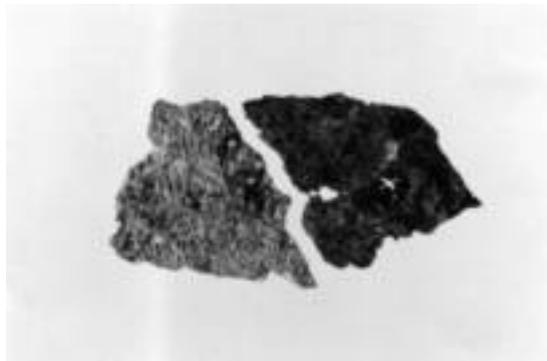
Figure 3 Copper alloy before (left) and after (right) plasma treatment.
